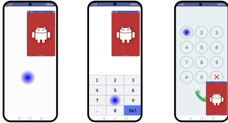
Figure 10: The experiment settings for IMU-based tap inference. Left: the tapping localization. Middle: the digits classification with a keypad at the bottom. Right: the digits classification with a keypad in the middle.
